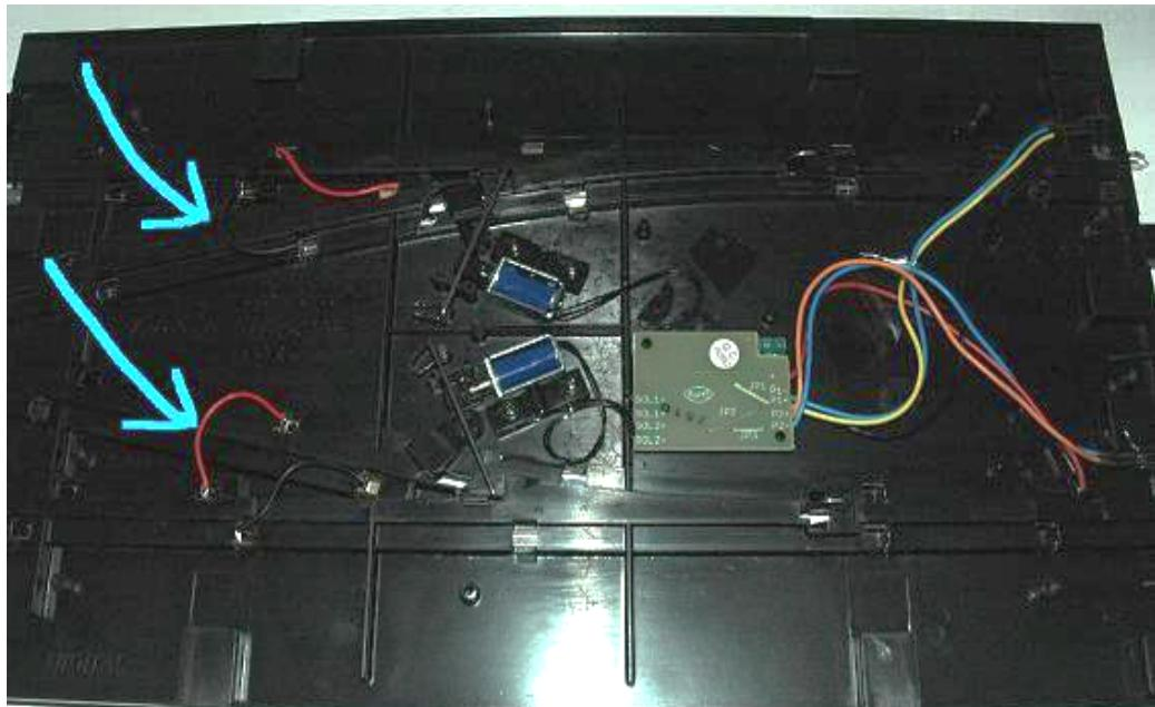
3. The numbers on the right side of the picture help identify each of the track rails. The factory red (+) wire needs to be located in rail #1. If it is in rail #3, move it to #1. The factory black (-) wire must go to rail #4. If it is in rail #2, move it to rail #4. In the image below, both of these wires need to be moved.
